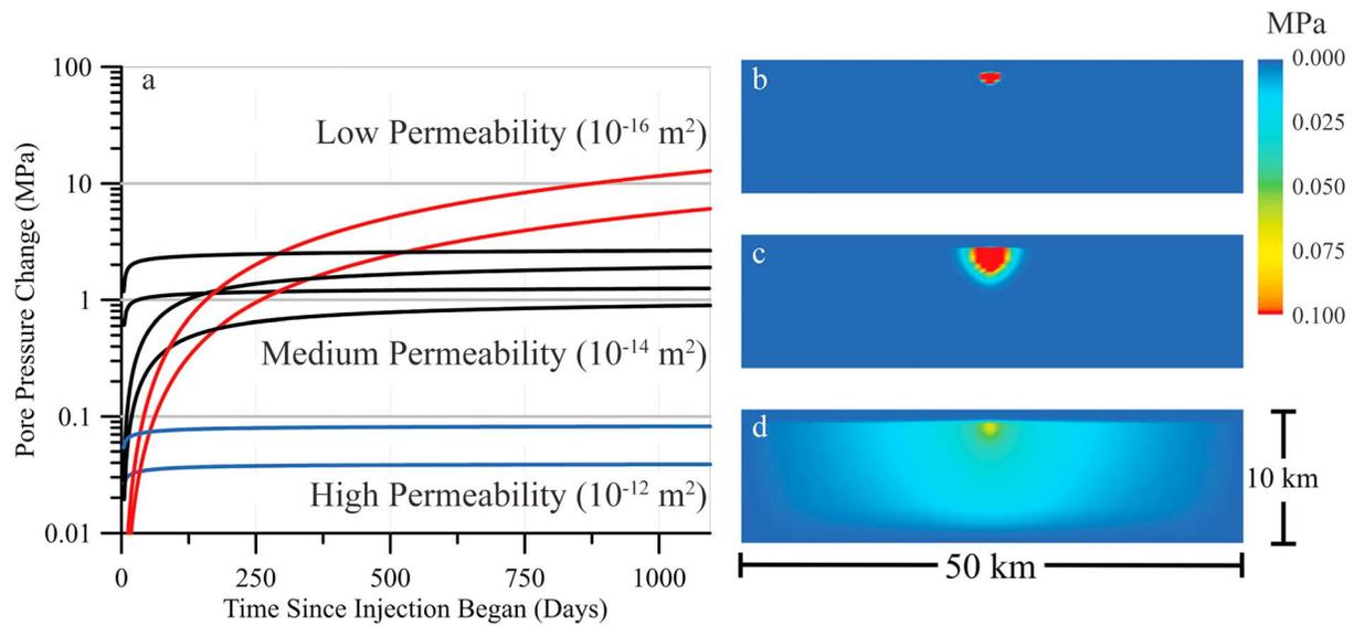
**Figure 2.** Pore pressure modeling results. (a) Graph of  $\Delta P$  at the yellow dot, shown in Figure S1a, directly below the injection well in crystalline basement. Simulations are grouped by permeability of injection interval (low, medium, or high). (b–d) Cross sections of  $\Delta P$  through the injection well after three years (1,095 days) of constant injection. (b) Low permeability, (c) medium permeability, and (d) high permeability.
